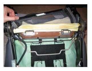
NOTE: The section by the airbag is tricky because instead of a clip, there is break-away material that is secured with two hog rings. Carefully un-bend these rings, and fold the material back:
