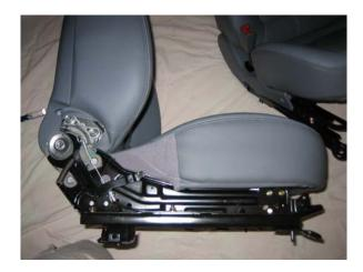
5. Flip the seat over, and with a quick pull, un-snap the bottom half of the plastic seatback and lift it off:
