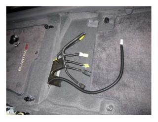
At this point, it is important to note that there is a distinct "RIGHT" and "LEFT" side to the wiring harness (the larger switch connection is for the "LEFT"). Examine the wire colors, and make sure you run the correct seat harness end to the correct seat.
