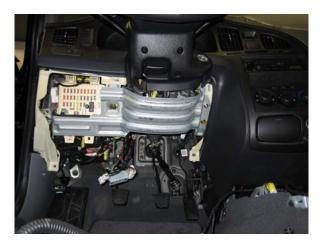
5. With everything now exposed, encase the seat harness end in the flex loom, and run it under the carpet along side of the other electrical connections:
