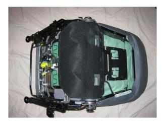
7. Starting with the upper seat cushion, unclip the long plastic clips holding the upholstery to the seat and fold the material back:
