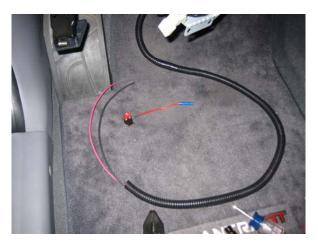
10. Connect the ATG fuse tap to the 12V power wire, and run everything up to the fuse box. One of the 10mm bolts for the steel shroud can be used as a ground:
