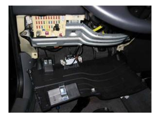
NOTE: There are a total of four Phillips screws holding the hood latch and diagnostic port to this panel. These will also need to be removed.
