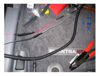
9. Stuff everything into the flex loom, leaving enough wire to work with at the end. Get the ATG fuse tap, and put the equivalent of 20amp fuses in it (1x20, 2x10, etc...):
