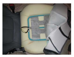
13. Following the reverse of the instructions above, reattach the seat upholstery and all of the plastic trim pieces. Be sure to leave the longer wiring connection accessible (but hidden behind the black felt).
