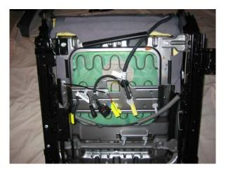
9. The upper seat upholstery is attached with Velcro. Carefully peel it back:
