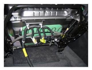
Some of these are easier to disconnect than others. Use the very small flat screwdriver, and <u>TAKE YOUR TIME</u>. One of these connections is spring-loaded, but with some very careful prying, it will also disconnect:
