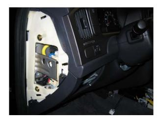
3. Using a 10mm ratchet, remove the two bolts as the bottom of the dash panel, and carefully pry it off (there are four clips on the upper panel):
