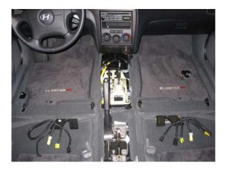
3. Get the OEM Hyundai parts. Install the rubber pad in the base of the tray. Install the switches in the console switch plate. Screw the switch plate to the underside of the tray.
