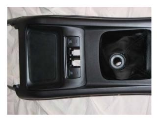
5. Installation of the console is the reverse of the remove – but don't do it yet - there's electrical work to be done!
