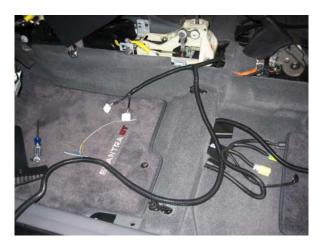
7. Take the flex loom containing the six free wires, and run this up towards the gas/brake pedals:
