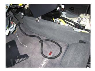
8. The longer white wire is the ground. Butt this to the 14gauge black wire, and seal it with heat-shrink tubing. The shorter white wire and the remaining four color wires are all 12V power. Butt them all together to the 14-gauge red wire, and seal it with heat-shrink tubing.
