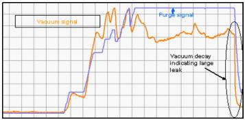
• The third check performed is the P0442 (Small Leak Detect). This diagnostic follows the same process as the Large Leak Detect described above, however, the threshold values are reduced. If a leak in excess of a 0.040" hole is detected, then DTC P0442 is set.
