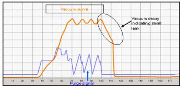
• The fourth check performed is the P0456 (Very Small Leak Detect). This diagnostic follows the same process as the two Leak Detect checks described above, however, the threshold values are the lowest. If a leak in excess of a 0.020" hole is detected, then DTC P0456 is set.
