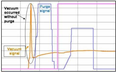
If the system failed the above PCSV DTC P0441 test, then a supplemental diagnostic check will be performed which checks for P2422 (Vent Path Restricted). This diagnostic is accomplished by opening the normally-closed purge valve and monitoring the fuel tank pressure sensor for an increase in vacuum. If the measured vacuum exceeds the threshold, then DTC P2422 is set to indicate a vent system restriction. (In some systems, P0446 may set instead.)
